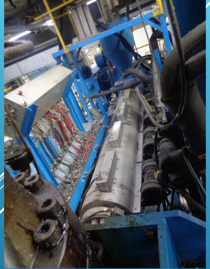
Extruder with material hopper
